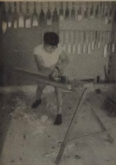
The angled planing beam is the most important bench in the workshop. The beam is supported in the front by a thin, three-slat trestle, and in the back by a short post propped against the wall.
